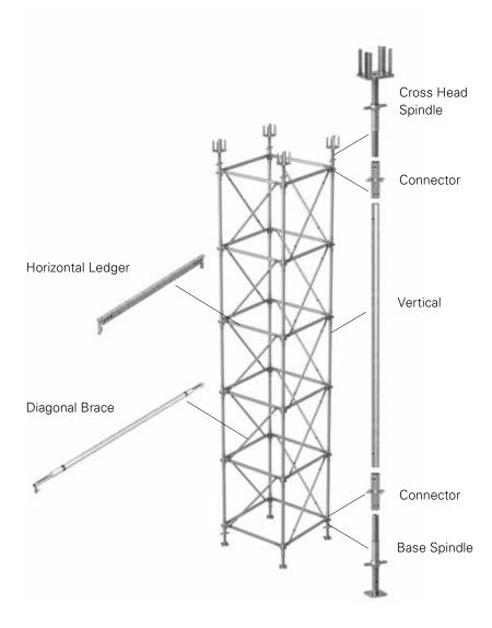
The system includes the innovative Connector MD, verticals and PERI UP ledgers and braces, supplemented with cross head and base spindles for continuous height adjustments. Thanks to its modular design and low number of system components, minimal storage space is required. At the same time, the PERI UP Shoring Tower MD can be easily adapted to different building geometries and a wide range of applications.
